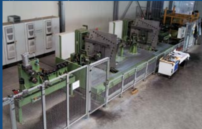
Blankdrahtwalzanlage copper bare wire rolling
